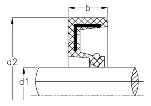
$\begin{array}{ll} b & = 12 \\ d1 & = 105 \\ d2 & = 140 \\ Material = NBR \end{array}$
